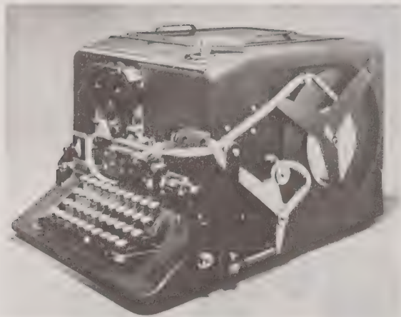
Figure 11: M-134-C (SIGABA) cipher machine used by the United States during World War II.
